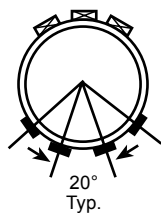
Figure 5-6 Typical skid arrangement
